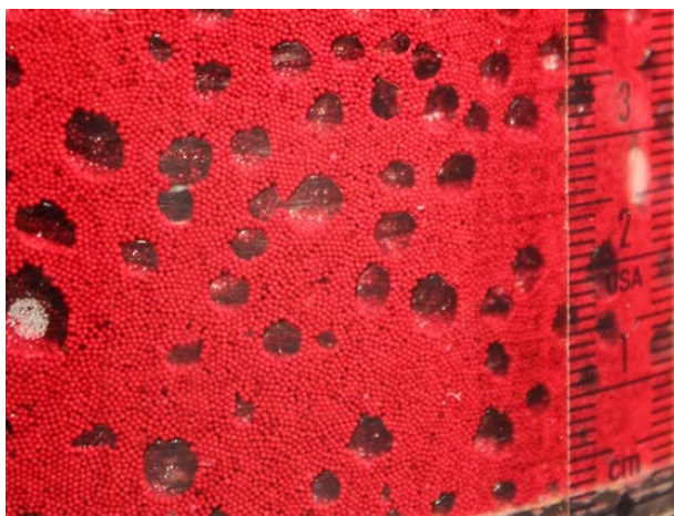
Fig. 8. Image of Hydrogen Gas Bubbles Generated Using Sodium Borohydride and Retained in a Bed of sRF Resin.
